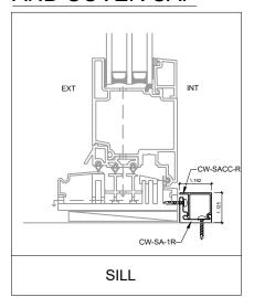
FLASHING ATTACHMENT ANGLE &
