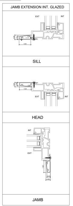
NOTE: THIS DRAFT DETAIL IS FOR GENERAL ARRANGEMENT PURPOSES ONLY, AND DOES NOT NECESSARILY REPRESENT A DETAIL THAT IS APPROPRIATE FOR A SPECIFIC PROJECT. PRODUCTS AND ACCESSORIES PROVIDED BY CASCADIA MUST BE CONFIRMED FOR SPECIFIC PROJECTS.
