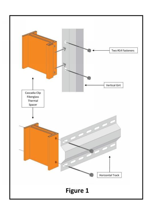
Figure 1. Cascadia Clip Typical Installation Details
