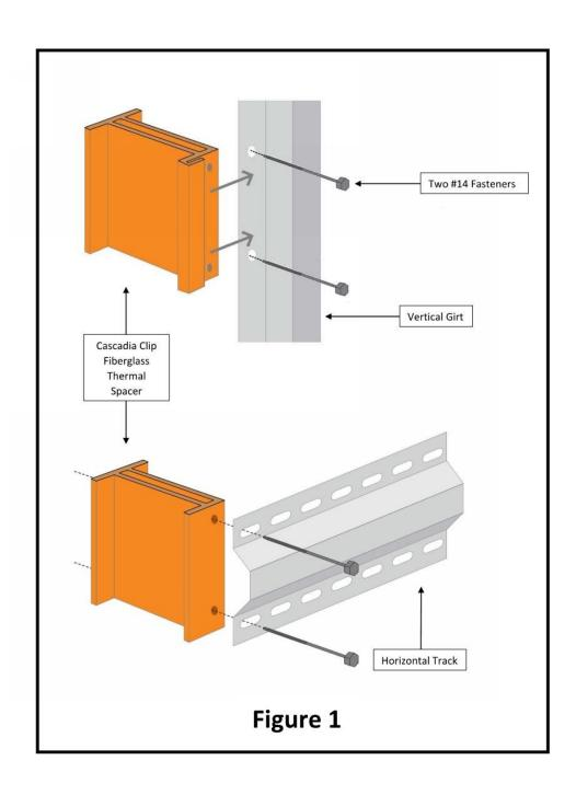
Figure 1. Cascadia Clip Typical Installation Details
